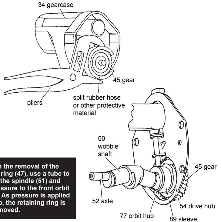
**To help in the removal of the retaining ring (47), use a tube to slip over the spindle (51) and apply pressure to the front orbit cap (59). As pressure is applied to the cap, the retaining ring is easily removed.**
