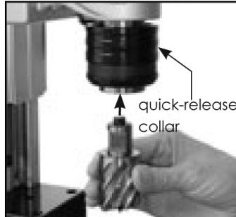
**Caution:** Never use a cutting tool that is larger than the maximum rated capacity of the machine.
