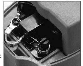
The brush design stops the machine before the carbon brushes are finished and protects the motor. In the event of the machine coming to a stop without obvious reason - then check the brushes immediately.
