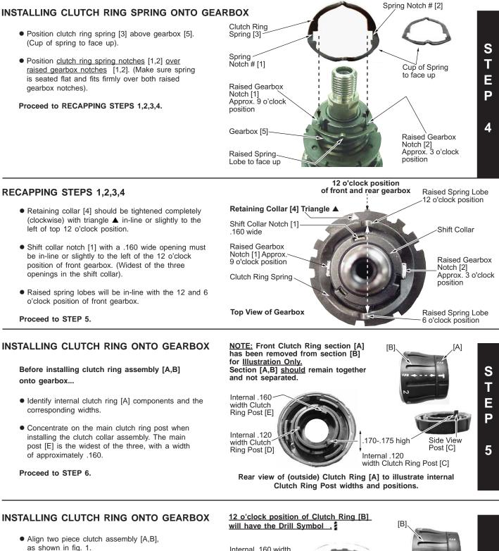
Turn clutch ring assembly to position shown in fig. 2 to view internal clutch ring posts [C,D,E] for correct position prior to assembling clutch ring to gearbox.
