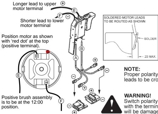
Proper polarity in the terminal block requires leads to be crossed as illustrated.
