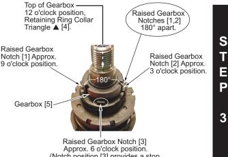
(Notch position [3] provides a stop for the .170-.175 long clutch ring post). 3
