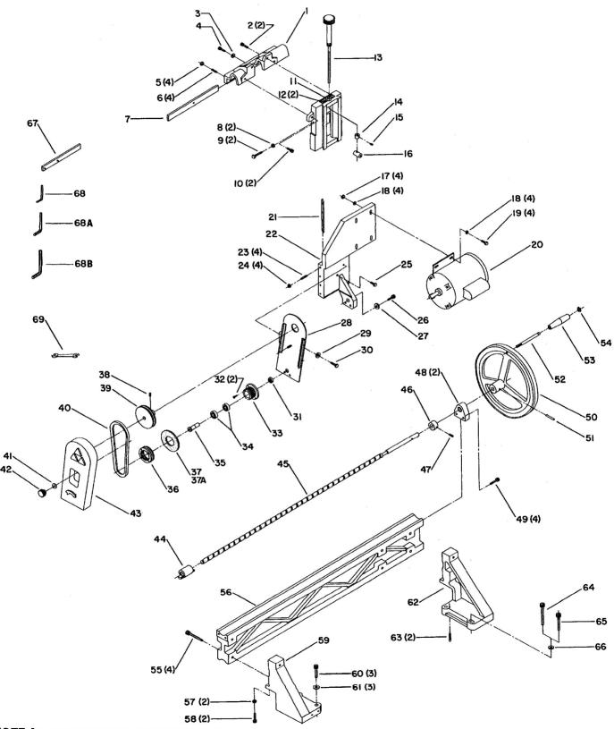
NOTE A: UNITS WITH SERIAL NUMBERS AS FOLLOWS, RC-63N - LOWER THAN 30, RC-63D - LOWER THAN 182, RC-51 - LOWER THAN 688 HAVE ADAPTER PLATES ON TOP OF THE LEFT AND RIGHT HAND BEARING BLOCKS WHICH REQUIRES THE USE OF A LONGER (80MM) MOUNTING BOLT AT THIS LOCATION ONLY.
