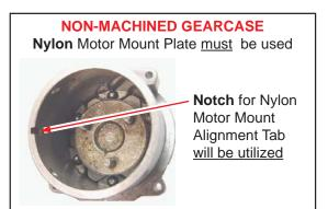
ASSEMBLY nylon motor mount with the original aluminum before
