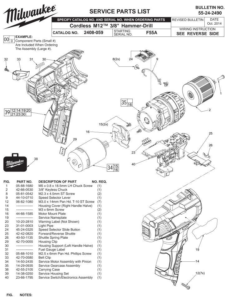
16,34,35 Service replacement gearcase assembly (35) comes with a motor mount plate (16) that must be removed and discarded when servicing. A motor mount plate already exists on the motor assembly (34).
