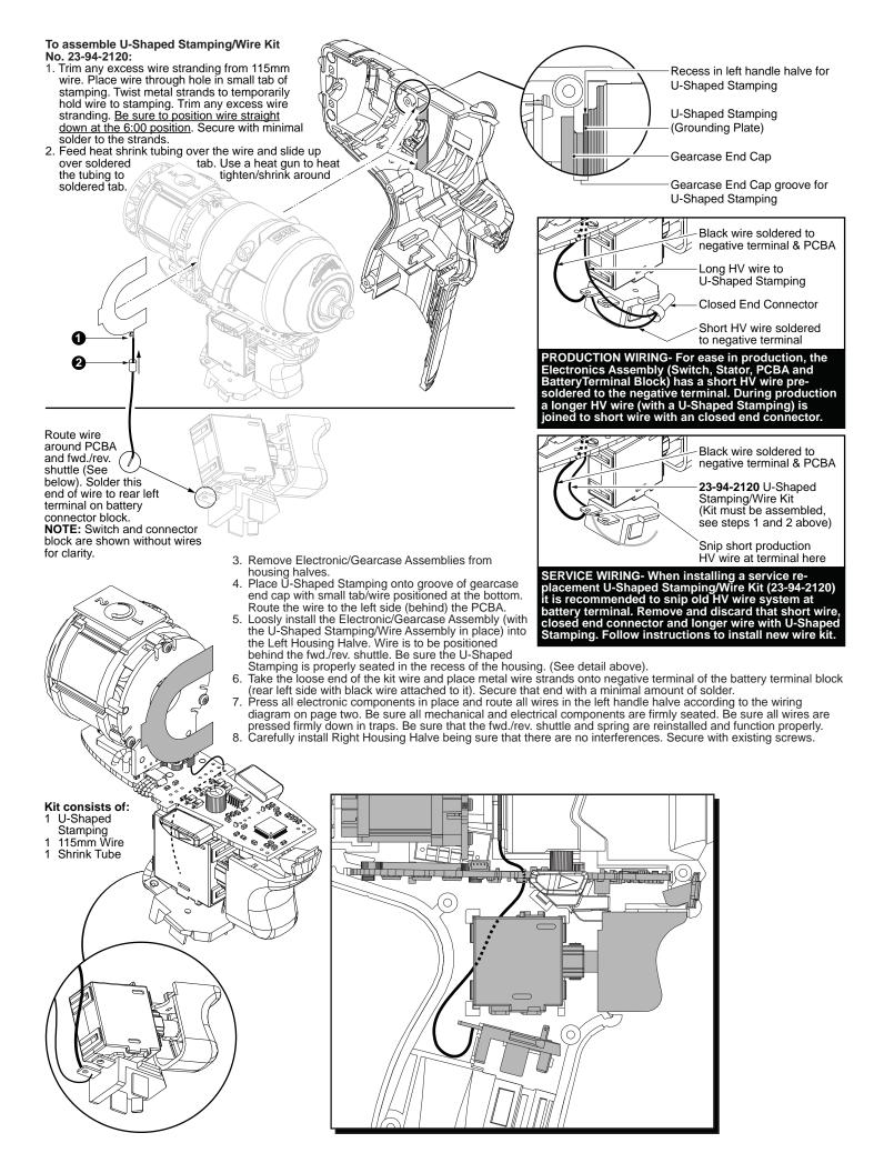
AS AN AID TO REASSEMBLY, TAKE NOTICE OF WIRE ROUTING AND POSITION IN WIRE GUIDES AND TRAPS WHILE DISMANTLING TOOL.
