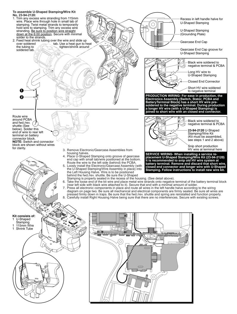
AS AN AID TO REASSEMBLY, TAKE NOTICE OF WIRE ROUTING AND POSITION IN WIRE GUIDES AND
