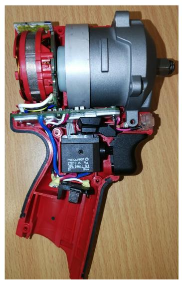
**STEP 11:** Assemble the gear case assembly onto the left housing halve and secure with two gear case screws.
