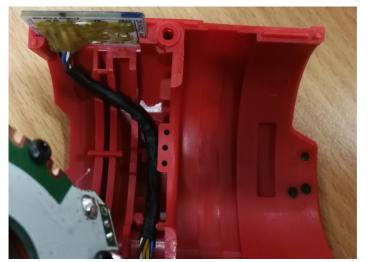
**STEP 5:** Install the pop switch into housing halve as shown. Route wires through traps being sure wires are tucked completely down.
