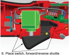
Place switch, forward/reverse shuttle and trigger in handle support recesses as shown
