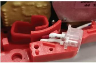
4. Place LED light in recess with the red wire to the top
