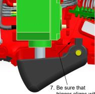
trigger aligns with rib as shown
