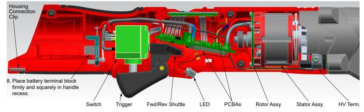
Prior to installing the Housing Cover, be sure all elements of the Electronics Assembly are seated properly (Stator, Main PCBA, Selector PCBA, On-Off Switch, LED Assembly and Battery Terminal Block Connector). Be sure the Grounding Terminal is in place and that all wires are pressed down into all wire traps and channels. Check to assure that
