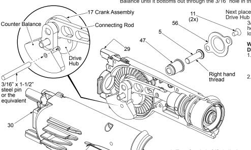
Next place a 3/16 hex key into Drive Hub Bolt (5) and turn Drive Hub Bolt slowly in a counter-clockwise direction until
