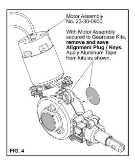
Install spindle / gearcase bushing assembly into right gearcase (coat components with type "L" grease and make sure spindle lock pin hole faces right gearcase). Note: If new felt seal is being
