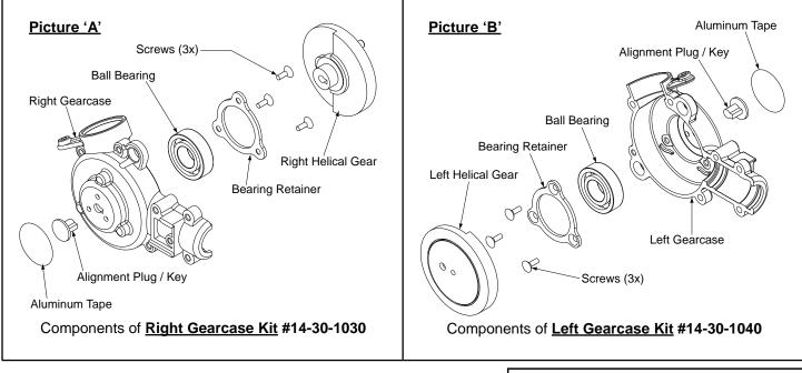
Picture "A and B" show the components that make-up the Right and Left Gearcase kits for M18 Cordless Hackzall 2625-20. Each kit contains one [1] Alignment Plug / Key and [1] round Aluminum adhesive backed disc (not sold separately) which will be needed when servicing / replacing the gearcase assemblies of the M18 Hackzall.
