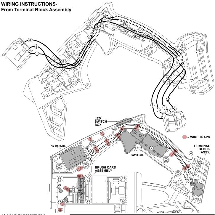
AS AN AID TO REASSEMBLY, TAKE NOTICE OF WIRE ROUTING AND POSITION IN WIRE GUIDES AND TRAPS WHILE DISMANTLING TOOL.
