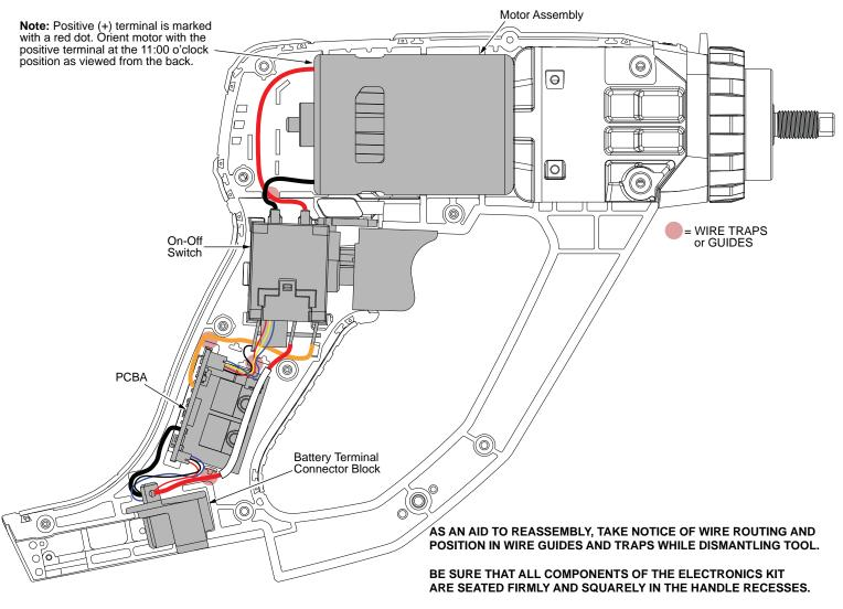
AVOID PINCHED WIRES, BE SURE THAT ALL WIRES AND SLEEVES ARE PRESSED COMPLETELY DOWN IN WIRE GUIDES AND TRAPS.
