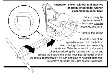
SERVICE TOOLS: Spreader Wrench No. 61-30-0300 for 14 Gauge Shear Head 48-08-0505 used on Shear No. 2636-20
