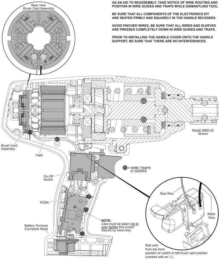
Black wire from top rear position on switch to right brush card position (marked with an 'R').
