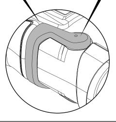
Place the tool on its side on a hard flat surface. Place a small wood block approximately 1-1/8' thick under the tool, between the hard surface and the shoe release lever, directly beneath the pin.
