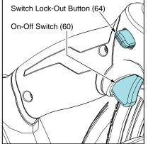
Functionally check Switch Lock-Out (64) by attempting to turn on tool by applying a reasonable amount of force, up to 8 lbs., to the switch trigger (60). The tool must not turn on.
