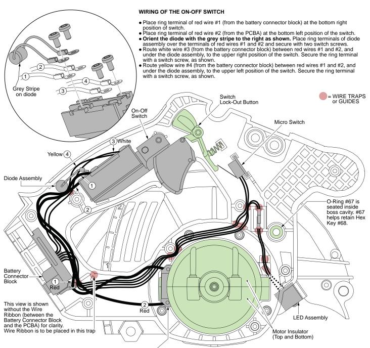
Stator / Electronics Assembly (Encased in the Motor Insulator Halves) Containing: Stator, PCBA, Battery Connector Block and Micro Switch
