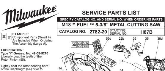
installing rotor (55).
