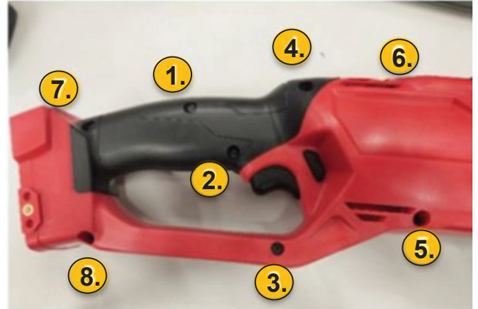
Step 6. Assemble Handle Halves together and secure with screws in the sequence shown above.
