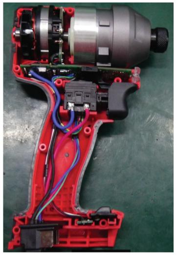
**STEP 10:** Check that all elements of electronics assembly are seated properly and that all wires are pressed completely down in wire traps and channels.
