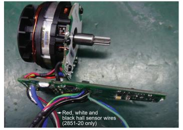
**STEP 1:** Carefully insert rotor into stator. Arrange wires as shown above. Note the red, white and black wires to the back of PCBA are connected to the hall sensor, model 2851-20 only. 2850-20 won't have the hall sensor.
