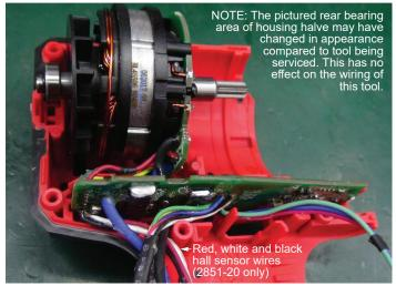
**STEP 2:** Place rotor/stator and PCBA firmly and squarely in cavities of left housing halve. Arrange wires as shown above.
