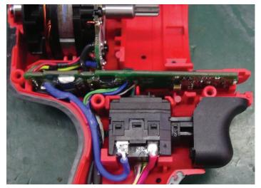
**STEP 5:** Place on-off switch firmly and squarely in cavity of left housing halve. Be sure all previously placed wires are still captured in properly in wire traps and channels.
