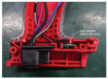
**STEP 6:** Place battery terminal block and hall sensor firmly and squarely in cavity of left housing halve. Be sure to capture hall sensor wires in trap as shown, model 2851-20 only.
