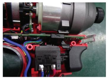
**STEP 8:** Install shuttle onto on-off switch being sure that top switch tab is captured in the bottom cavity of shuttle. Check for proper shuttle and switch functionality. Install LED lens into housing halve recess.
