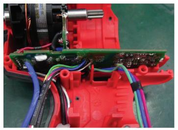
**STEP 3**: Separate and organize wires as shown above. For the 2851-20, place three hall sensor wires in bottom of housing halve behind on-off switch cavity. Place black battery terminal wire over those three wires.
