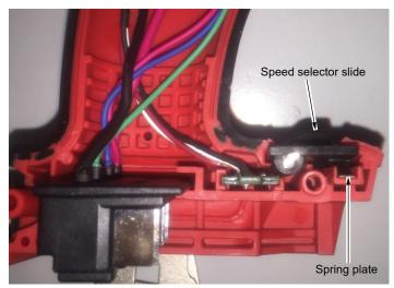
$\ensuremath{\textbf{STEP 9:}}$  Install spring plate and speed selector slide into left housing halve.
