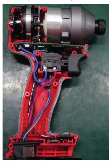
**STEP 10:** Check that all elements of electronics assembly are seated properly and that all wires are pressed completely down in wire traps and channels.
