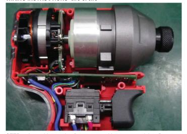
**STEP 7:** Assemble gear box/impact assembly onto rotor pinion. Be sure gear box, rotor and stator are firmly and squarely seated in left housing halve and that the rotor fan has movement.
