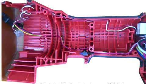
Prior to installing the electronics assembly into the housing support, place grounding terminal over screw boss as shown. Route ground wire, removing as much slack as possible. Be sure wire is pressed firmly to the back of the wire traps.
