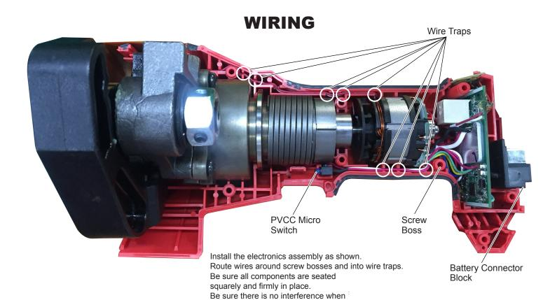
installing the housing cover.
