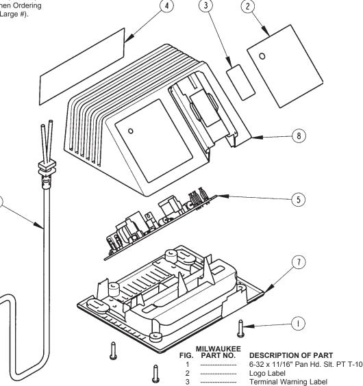
Rib of top housing is to separate the terminals of circuit board assembly and the cord set wires.
