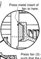
Press fan (3) onto armature (30) such that the metal insert of the fan bottoms against the fan journal shoulder of the armature shaft.
