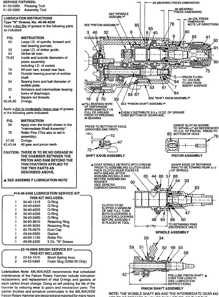
NOTE: THE WOBBLE SHAFT #59 AND THE INTERMEDIATE GEAR #42 ARE TO BE PRESSED FLUSH TO EACH OTHER, SO THAT THE WOBBLE SHAFT IS STILL ABLE TO REVOLVE FREELY - WITH .005" MAXIMUM AXIAL PLAY ON THE INTERMEDIATE SHAFT #43.
