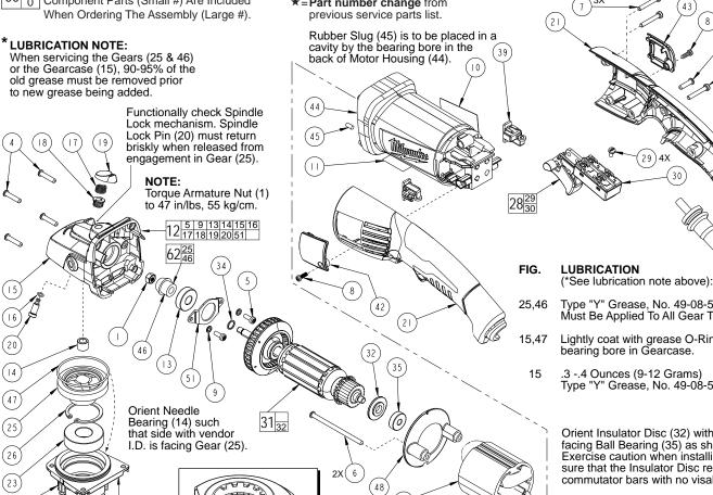
Type "Y" Grease, No. 49-08-5270, Must Be Applied To All Gear Teeth.
