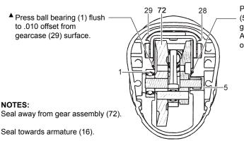
Press needle bearing (5) flush ± .010 from gearcase (28) surface. Apply Green Loctite 620 or equivalent.
