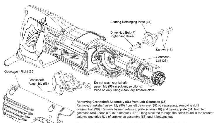
Next place a 3/16" hex key into drive hub bolt (7) and turn drive hub bolt slowly in a counter clockwise direction until 3/16" steel pin rest against crankshaft assembly connecting rod. The 3/16" hex key can now be forcibly turned counter clockwise to loosen and remove drive hub bolt (7).
