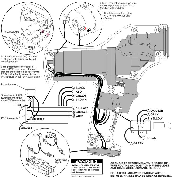
NOTE: Proper polarity in connector block requires leads to be crossed, as illustrated.
