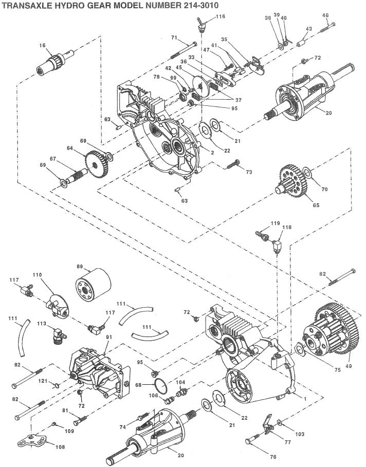
20 HP 50" TRACTOR - MODEL NO. GTH200 (HN20H50A), PRODUCT NO. 954 00 06-82 TRANSAXLE HYDRO GEAR MODEL NUMBER 214-3010
