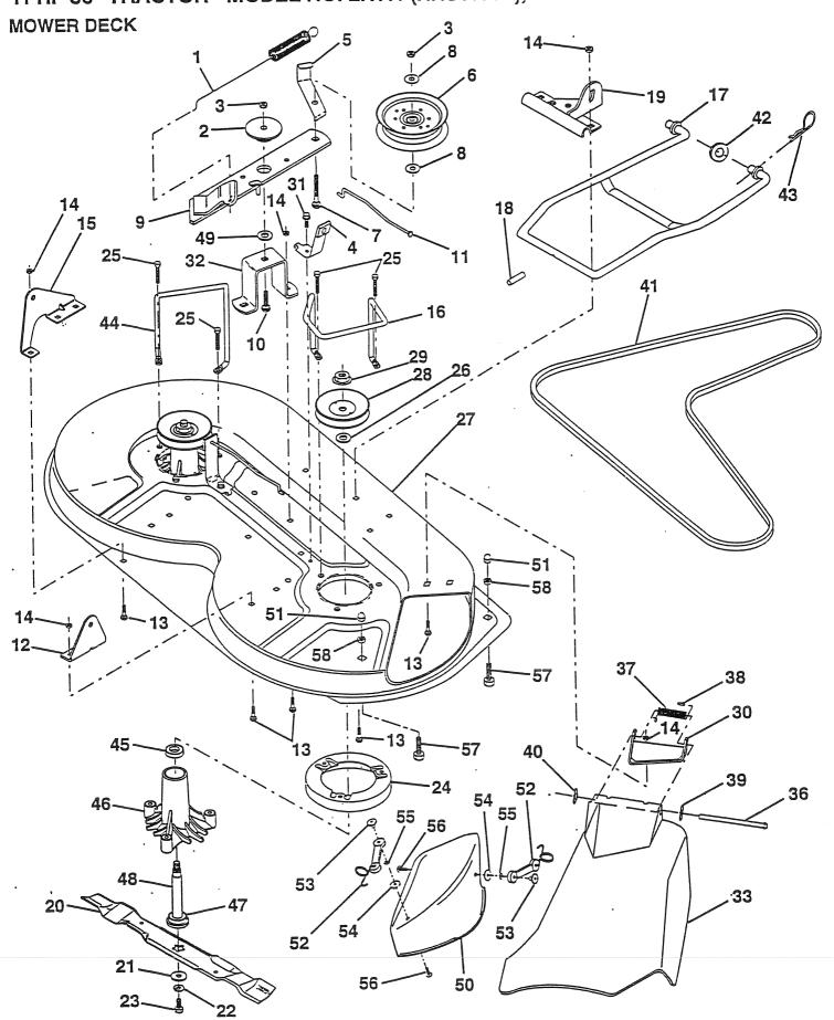
11 HP 36" TRACTOR - MODEL NO. LR111 (HNS1136A), PRODUCT NO. 954 00 06-32 MOWER DECK
