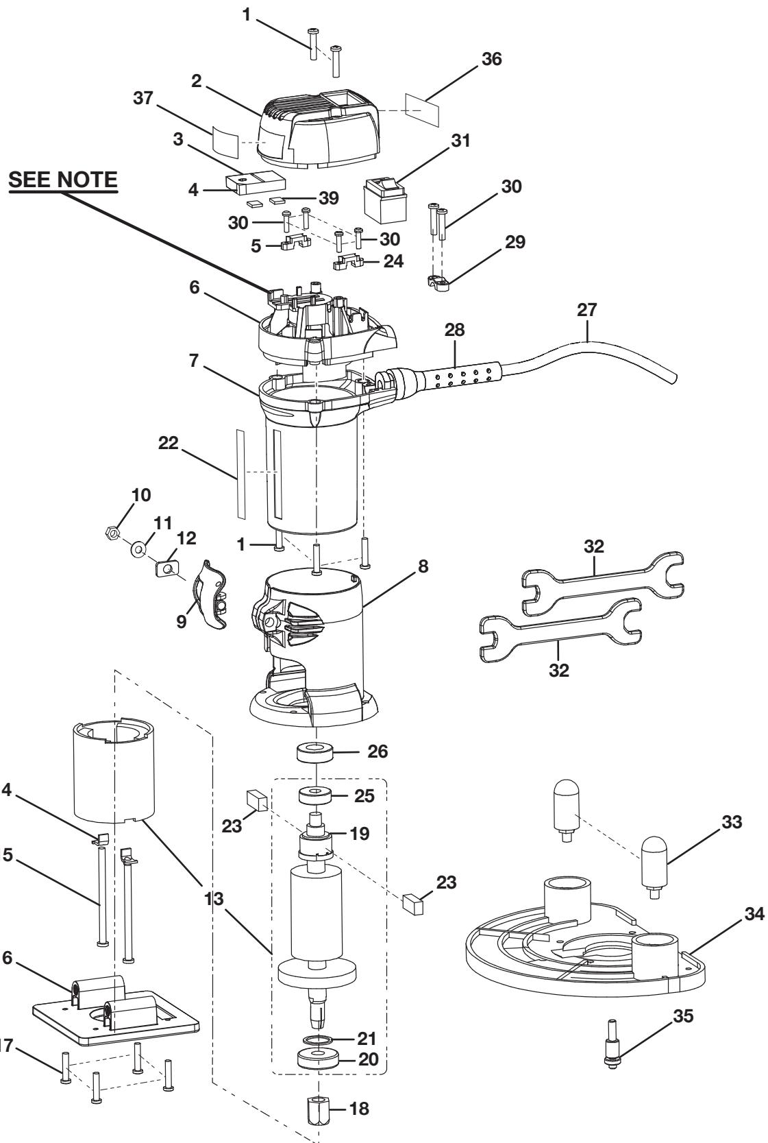
**NOTE: THE ASSEMBLY SHOWN REPRESENTS AN IMPORTANT PART OF THE DOUBLE INSULATED SYSTEM. TO AVOID THE POSSIBILITY OF ALTERATION OR DAMAGE TO THE SYSTEM, SERVICE SHOULD BE PERFORMED BY YOUR NEAREST RYOBI REPAIR CENTER.**
