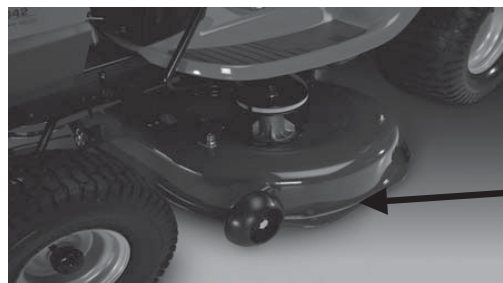
Stamped Deck Shell below, NOT reinforced
