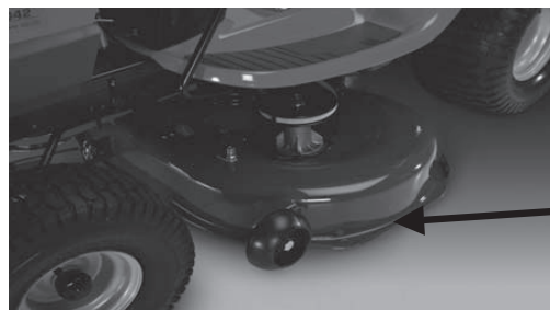
Stamped Deck Shell below, NOT reinforced
